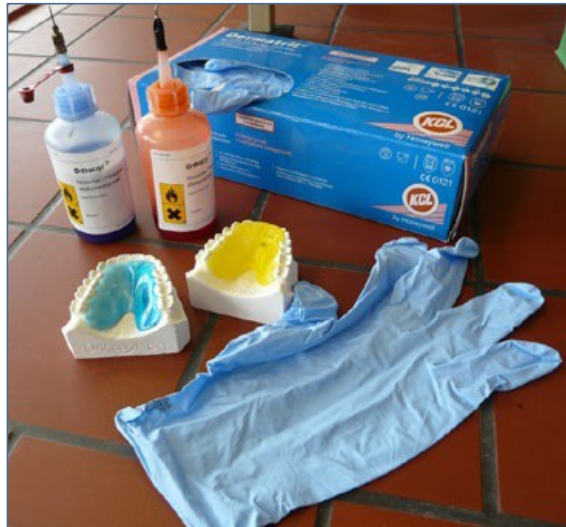
Fig. 13 When processing MMA, direct skin contact must be avoided by wearing suitable gloves.
