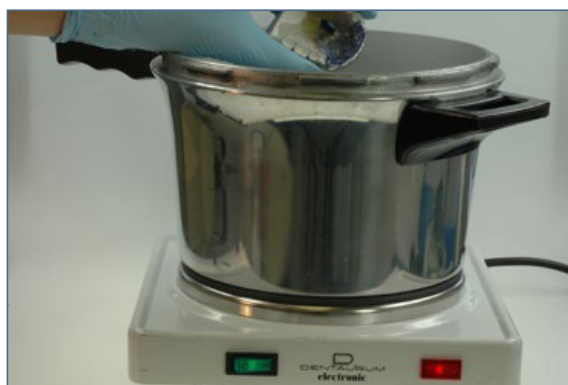
Fig. 10 A heating plate allows the water in the pressure vessel (Polyclav, Dentaureum) to be kept constant for the entire polymerization period.
