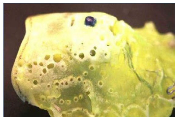
Fig. 11 Bubble formation in the acrylic due to processing errors. The model was not watered and boiling bubbles appeared.
