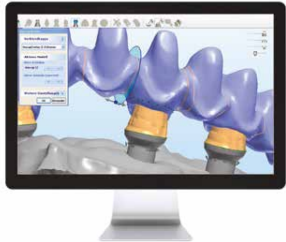
Framework design in CAD/CAM software.
