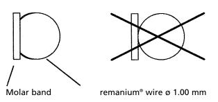
Larger gaps can be filled with remanium® wire Ø 0.35 mm (REF 535-035-00) as a filler material. First, the 0.35 mm wire is welded to the band and then to the 1.00 mm wire (Fig. 3).
