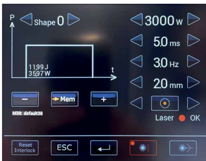
Figure 14: Touchscreen main window – in save parameter set mode
