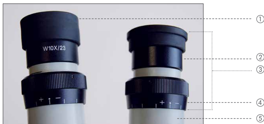
Figure 17: Ocular and eyecups of the standard microscope attachment
