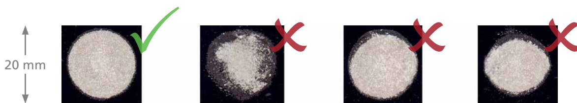
Figure 26: Focal spot impression on photographic paper
