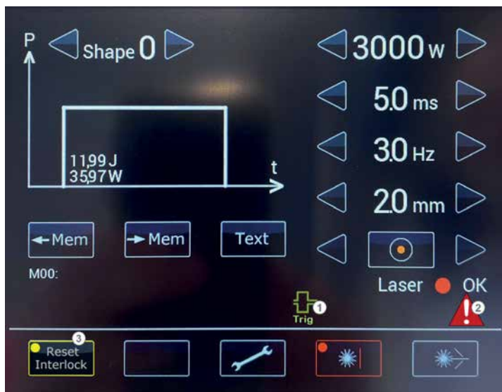
Figure 21: Touchscreen – error message (=interlock)
