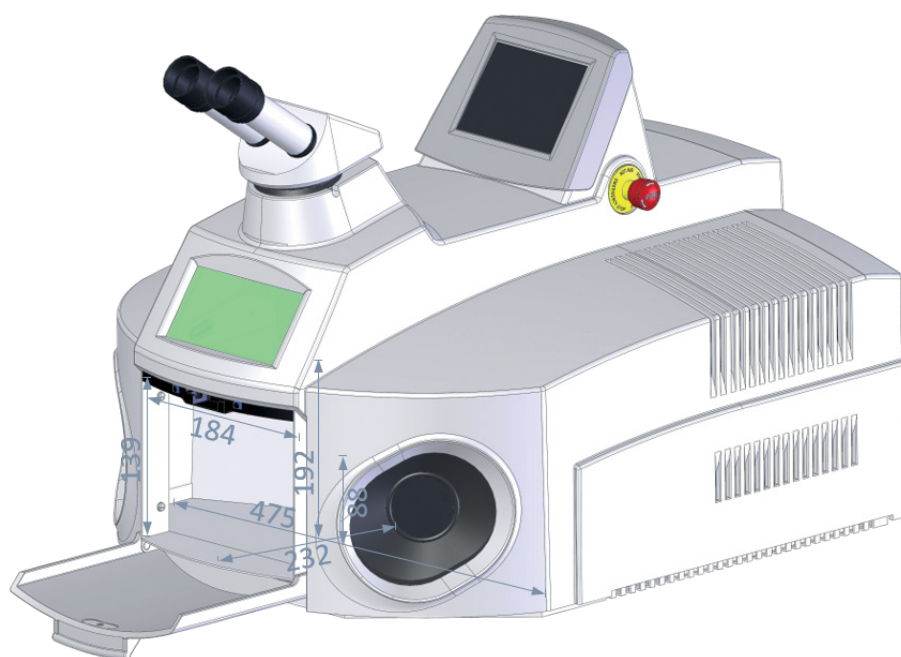
Figure 6: Working chamber dimensions
