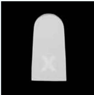
Fig. 5: underfired material sample
