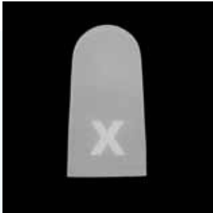
Fig. 4: correctly fired material sample
