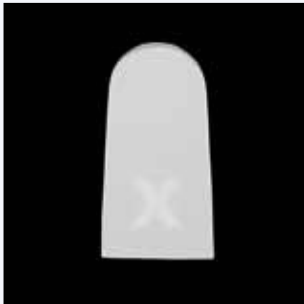
Fig. 5: underfired material sample
