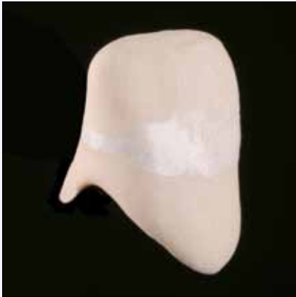
Fig. 4: Paste Opaque fired with inlaid white band
